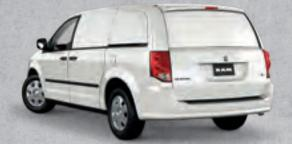
**SOLID FULL-WINDOW PANEL INSERTS.** The standard configuration for Ram C/V Tradesman features molded privacy inserts for both sliding doors, the rear-quarter vents, and the rear liftgate.
