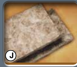
J Full 6 sided R-7 eco-batt insulation. This is a new and sustainable technology
