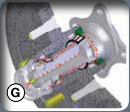
G Superlube™ axles for fast and easy lubrication
